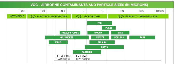
All centralised SmartVent systems feature high grade F7 filters that capture up to 90% of 0.4 microns particles such as fine pollens, dusts and allergen from the air making the air cleaner to breathe. High quality HEPA filters are also available for asthma and allergy sufferers.
